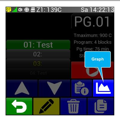
The selected program can also be displayed in graphic form. If the program is empty, this function (Graph button) is not available. After pressing the button (Graph) the following screen will appear:
