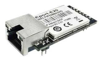
The CLARE 5 controller can optionally include an Ethernet module, which allows the controller to connect to a computer network and access some Internet services. The module is soldered to the processor board at the RS-485 output point. The RJ-45 connector is then placed instead of the terminals C1 - C4 (see the article <u>Konektory regulátoru</u>). In that case, the RS-485 communication output can no longer be used.
