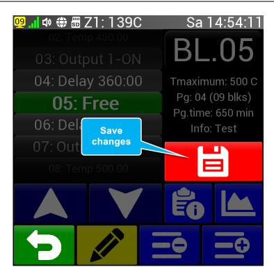
After modifying the program, it is necessary to save the program in the memory of the controller. This is what the button is for (Save), which is automatically displayed when a change is made in the program. After pressing this button, the changed program is saved and the button disappears. If we do not save the program, then the changes made will be lost in the following cases:
