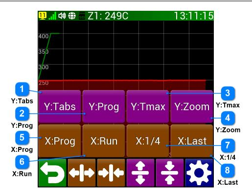
The graph settings bring predefined ranges of temperatures and times for faster display of the required graph scales. It offers 8 buttons, 4 for adjusting the temperature range and 4 for adjusting the time range.
