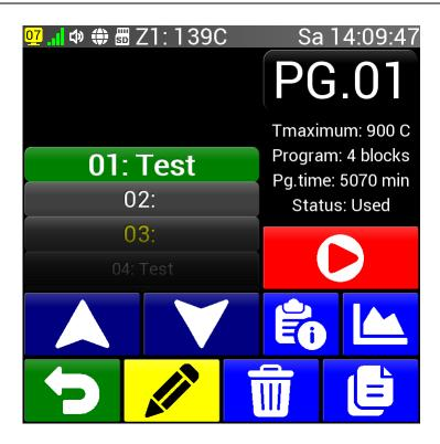
Programming mode allows incomparably greater variability than manual mode. Getting to know it will allow us to use most of the functions of the controller effectively. In the programming mode, even very complex thermal processes can be programmed, for example for weeks in advance.
