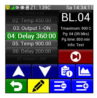
The screen for managing blocks is very similar to the screen for working with programs. Here we can select a specific block in the list of program blocks, enter a label and display the program graph, insert or delete a block, and last but not least, there is a button for editing the selected block or starting the program from a specific block. We will describe these functions in the following articles.
