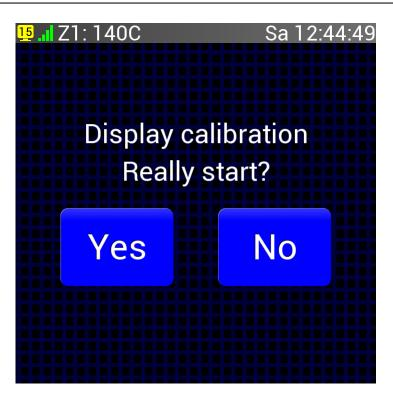
In case of inability to control the controller or inaccuracy during touch control, it is necessary to calibrate the display by pressing and holding the touch layer for 30 seconds. The hold needs to be done on the screen away from the places where the buttons or graph are. The screen below will then appear.
