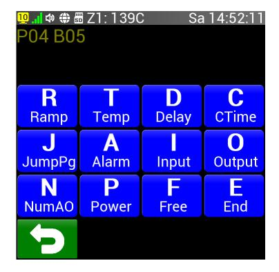
All the functions that the insertable block can contain are available on this screen. If we change our mind about inserting a block (another command), we can return to the previous screen using the button (Back). Otherwise, by pressing the appropriate button, we choose which command we
