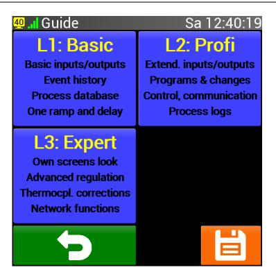
This screen appears in the Installation Wizard after entering the maximum temperature.
