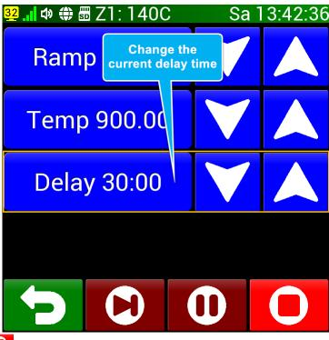
By pressing the button O (Stop) on the home screen while the program is running, we get to the screen for preparing to end the program. If the Settings (article <u>Changing the program on the fly</u>) allow changing the parameters of the program while it is running, we will see in the upper part of the screen the possibility of changing the current delay time at the set temperature (see upper picture).
