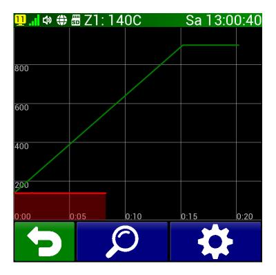
It shows an enlarged graph and a series of buttons. More information about controlling this enlarged graph is in the next article <u>Graph control</u>. Press the **S** (Back) button to return to the home screen..
