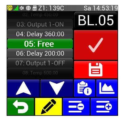
The button gradually disappears and after about 5 seconds it disappears and the program information appears again. If we press the button during these 5 seconds, the selected block will be deleted and all other blocks will have their number reduced by one.
