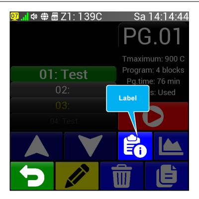
The program label is used to identify the program as well as its serial number. Each program can be marked with any text of up to 39 characters. The beginning of the program description can also be seen in the list of programs next to the program number. Therefore, it is advisable that the beginnings of the labels are different for clarity.
