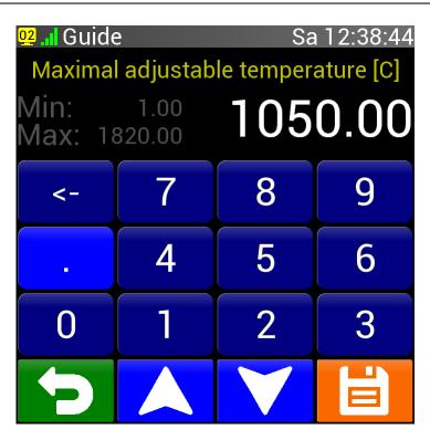
After selecting a thermocouple, a new screen will appear. In this step, you need to correctly enter the highest adjustable temperature for the connected device. This parameter will be provided by the documentation or manufacturer of the device. The value can be entered in two ways:
