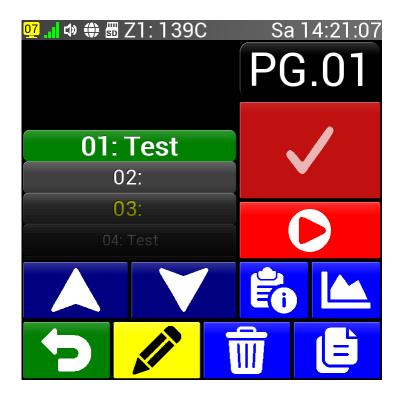
The button gradually disappears and after about 5 seconds it disappears and the program information appears again. If the button is pressed during these 5 seconds, the selected program will be deleted. The program can also be deleted by writing the command End in the first block of the program. The deleted program becomes empty (yellow font).
