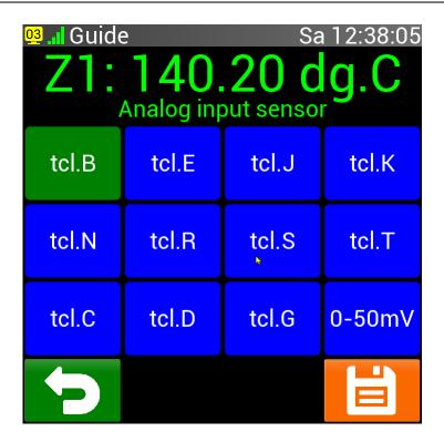
This screen will appear immediately after saving the date and time. At this stage of the wizard, it is necessary to select the type of thermocouple (marked on the terminal board as TC). The available types of thermocouples are: B, E, J, K, N, R, S, T, C, D, and G. Detailed information on thermocouples can be found in the appendix. Confirm the selected thermocouple with the diskette button in the lower right corner of the screen.
