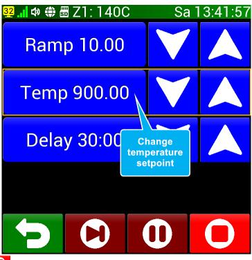
By pressing the button O (Stop) on the home screen while the program is running, we get to the screen for preparing to end the program. If the Settings (article <u>Changing the program on the fly</u>) allow changing the parameters of the program while it is running, we will see in the upper part of the screen the possibility of changing the current set temperature (see upper picture).
