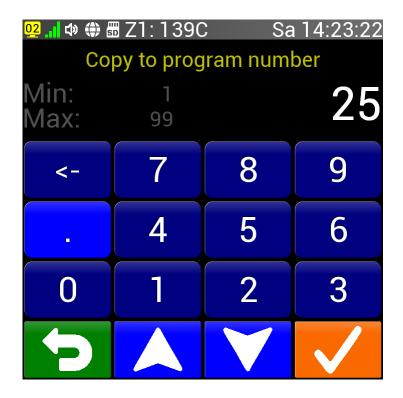
On this screen, we enter the program number (position) to which we want to copy the previously selected program. With a button (Back) we return to the previous screen without copying the program, it is actually canceling the copy operation. Button (OK) on the other hand confirms the copying and the program is copied to the specified position. At the same time, it returns to the previous screen and moves the list of programs to a new position. This will facilitate its possible
