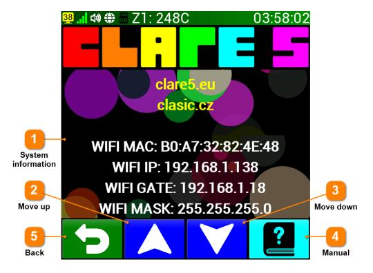
On this screen we can find information about the configuration of the controller, contact the manufacturer and enter the screen with the manual for the controller. The information is scrolled automatically, it is possible to speed up the display of others by moving your finger up / down or by pressing the appropriate buttons. Scrolling can also be paused or restarted by simply touching the information.
