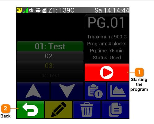
If we select a program that is not free (empty) in the previous article, a button to start the program will appear. If we do not want to start the program and want to leave the programming program, we use the button (Back). When using the button (Start) the following preparation screen for starting the program will appear:
