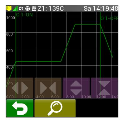
The graph plots the dependence of the temperature on the time of the selected program and displays important blocks in the program with vertical lines with a description. The graph can then be controlled in the same way as in the previous article <u>Graph control</u>. With a button (Back) we return to the selection (number) of the program.
