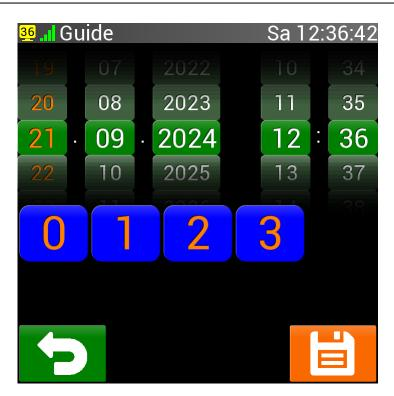
After pressing the button with the desired language, the following screen will be displayed. On this screen, you can set the current date and time. Values can be entered in two ways:
