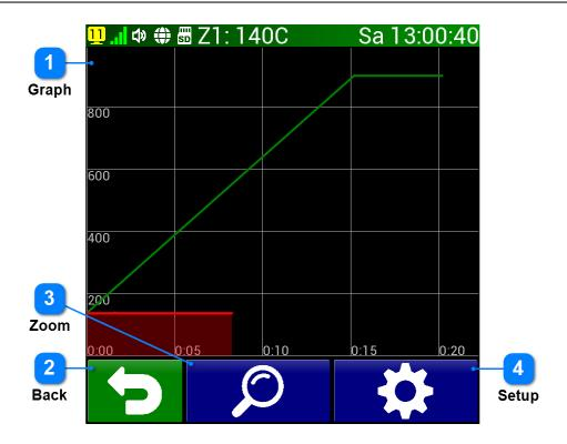
The graph screen is used to accurately display the programmed temperature curve and the current (or earlier, for waveform database) actual temperature curve. In the basic settings, the program curve is drawn in green and the actual temperature curve in red. The curves can be zoomed to a resolution of 0.01°C and 1 second. The graph can be moved by touch, enlarged, or the button bar can be used to achieve the desired graph display. This large graph screen will appear in the following cases:
